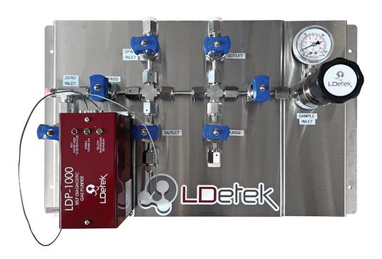
The LDGM gas manifold is used as an ultra high purity sampling system for any sensor or analytical device that requires switching between a zero gas, a span gas and the sample gas for calibration and proper analysis. The electropolished Stainless Steel 316L gas lines with the quarter turn on/off diaphragm valves guaranteed a quick analysis time without drifting at low ppm/ppb especially for trace analysis Nitrogen, Oxygen and Moisture.
