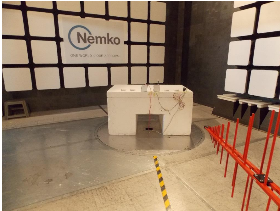
Figure 8.2-5: Radiated emissions setup photo – below 1 GHz
