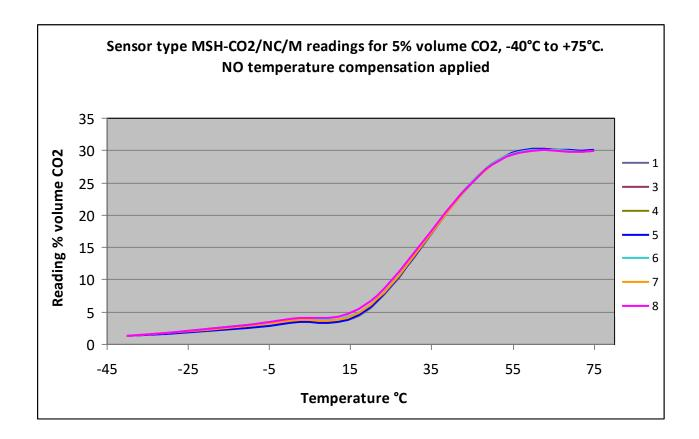
The non-linear nature of the span temperature dependency needs to be taken into account when applying temperature compensation. Whilst the variation from sensor to sensor is very small, multiple-point temperature compensations are required in order to achieve accurate results across the full operating temperature range.
