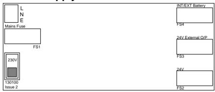
The Power Supply is situated beneath the main chassis of the control unit and provides the power for the whole system. The power supply is a standard item and does not require any modifications regardless of the type and quantity of detector heads being used.
