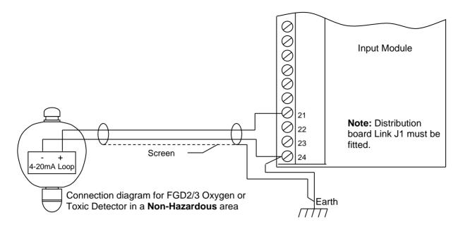
The correct wiring method for all Status Scientific FGD2 / FGD3 Detector Heads (in a non-hazardous location) is shown above. It is important to note that this drawing shows the wiring connections but does not discuss the Input Module configuration. Prior to connecting the Detector Head ensure the Input Module is correctly configured (refer to section **4.1**).
