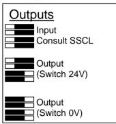
**Input** – Allows the outputs to be configured as inputs in some circumstances. Contact Status Scientific for further details.
