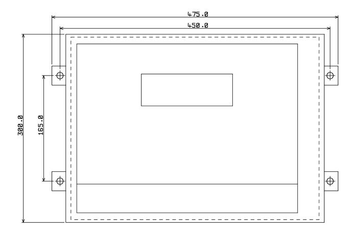
**Note:** The front panels of the MCU Control Units open to allow access to the screw terminals situated inside. Sufficient space should be allowed around the mounting position so that this action is not restricted.
