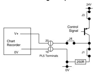
The SCM1 can provide a voltage output.
