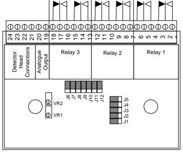
The relay connections shown are with the relay coil in its de-energised state.
