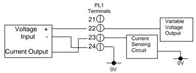
This configuration allows the connection of a detector head that provides a 4-20mA current output, and requires a separate power source, between 0-24V.
