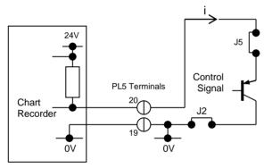
The Input Module can also sink current proportional to the detected gas level.
