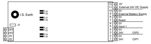
The lower 4-way connector provides two 24V screw terminals, and two 0V screw terminals. The voltages are always present at these terminals whilst FS3 is intact. This supply is taken from the 24V supply of the system and is used by Status Scientific Controls when powering external equipment. The amount of power available from this connector must be determined for each installation based upon the system configuration.
