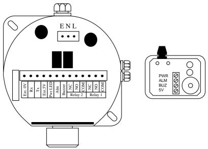
To gain access to the terminals within the remote indicator assembly, remove the screw located at each corner of the assembly when viewed from below (4 in total).
