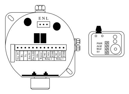
To gain access to the terminals within the remote indicator assembly, remove the screw located at each corner of the assembly when viewed from below (4 in total).
