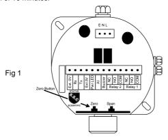
Ensure the sensor is in a zero-gas environment.
