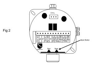
Apply a known concentration of gas (applicable to sensor type) at a flow rate of between 200 and 500cc/min. Allow time for the sensor to respond. Press the Span button and hold for a minimum of 5 seconds to span the sensor.
