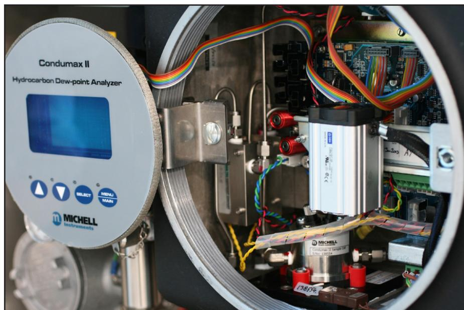
Figure 6 *Removal of Interface/Display*
