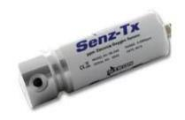
With a choice of either zirconia or electrochemical sensor technology the SenzTx offers reliability, accuracy, and flexibility. Both technologies have a broad measurement capability allowing the user to measure from selected ranges from 1ppm to 96% oxygen.
