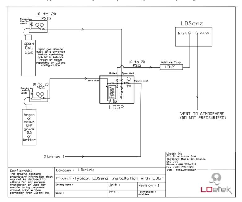
Typical installation using "LDGSS" gas multi-stream selector for Zero/Span/Samples
