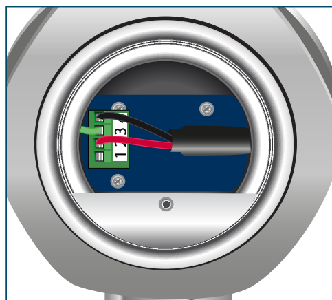
Figure 6 Terminal Block Connection
