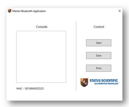
Providing that the device has native hardware Bluetooth or a Bluetooth dongle, the application should display the MAC address of the Bluetooth transceiver.
