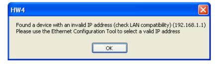
Use the Digi Device Discovery tool to change the TCP/IP settings of the device so as to make it compatible with the local area network.
